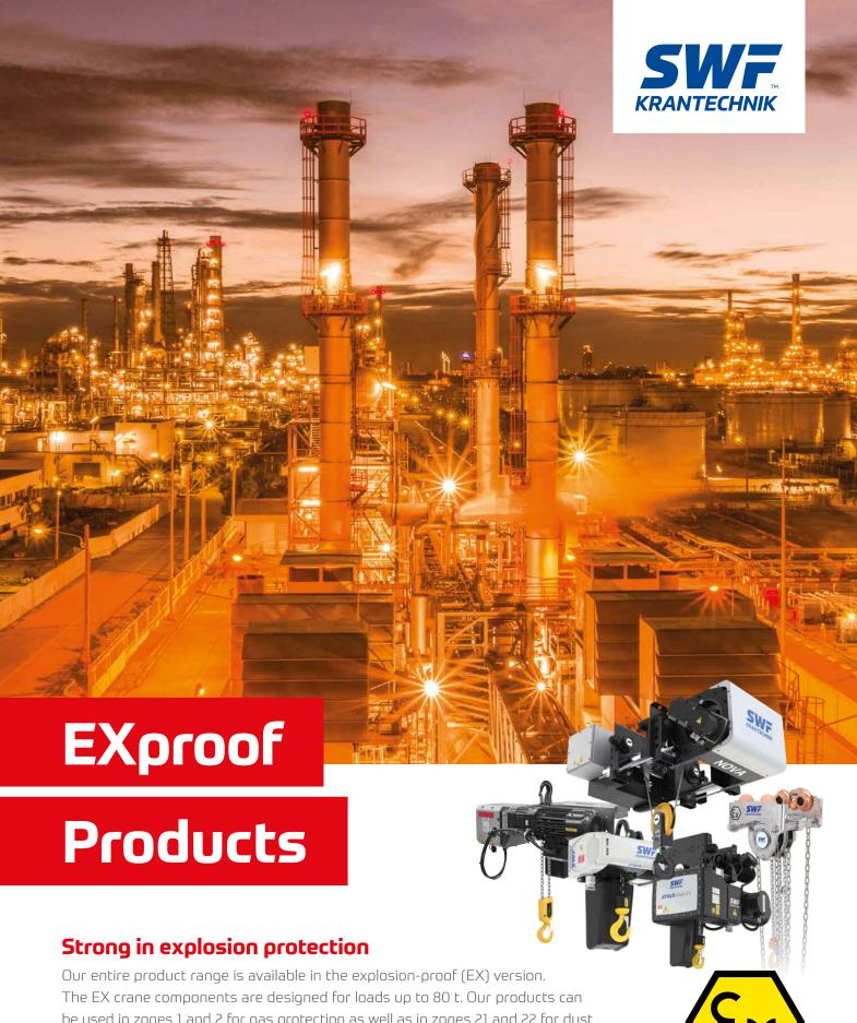
The EX crane components are designed for loads up to 80 t. Our products can be used in zones 1 and 2 for gas protection as well as in zones 21 and 22 for dust protection. They meet the highest European and international safety standards according to ATEX and IECEx. Our EX products are used in all industries and we have many years of expertise in the EX area.
